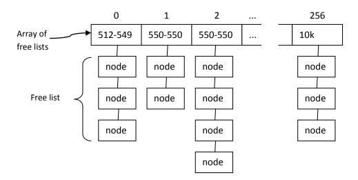
To allocate a specific size it first finds the free list, and then iterates over the nodes to find one that is big enough. If no nodes are big enough it tries the next free list. When a region is created it creates a single free block of the entire region size and adds it to the free list at index 256.
