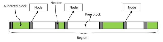
The reason that the free nodes are not embedded into the header is speed up iteration and sorting of the free lists. The nodes are all allocated using an internal FSA which makes iterating over the nodes very cache friendly.
