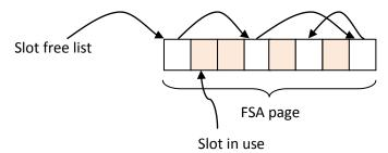
The FSA has a page free list which contains pages that are partially full. When a page is full it is taken off the free list and when a page is empty it is given back to the page heap. Each page has its own slot free list. The reason that the FSA has a page free list and free slot list per page rather than on single free slot list that spans all pages is because of the biasing.
