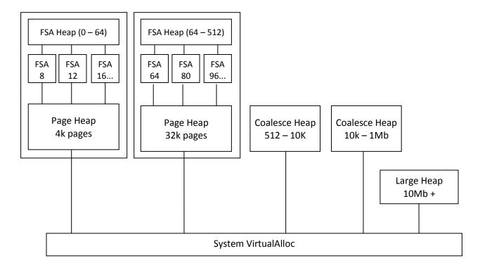
Additionally VMem has a basic FSA and a basic coalesce allocator. These allocators get the memory directly from the system and have no internal overhead. Overhead for the other allocators and heaps is allocated using these basic allocators.
